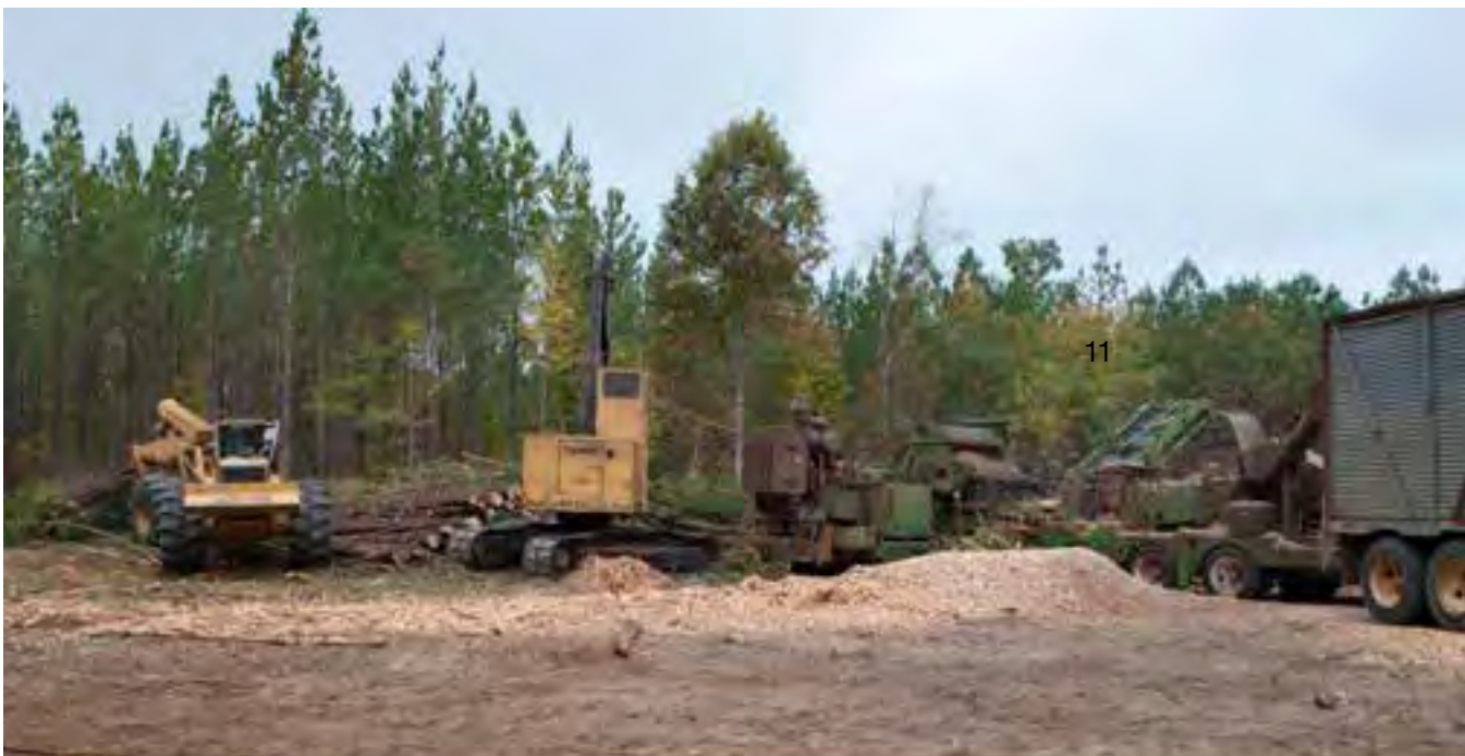
A skidder operator delivering trees at an in-woods clean-chipping operation featuring a loader, flail, disk chipper, and chip van.
